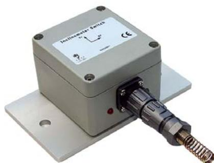
**NTI-T245-FDA** series is a two-axis inclinometer switch which is researched and produced for Nordic Transducer Denmark. The measuring range is +/- 45 degree. Switch trigger point can be set by ASCII command freely. It can be widely used in engineering mechanism field.
